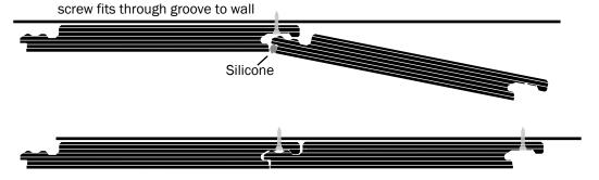
Silicone sealant should be applied to the tongue edge, then angled into the groove.
